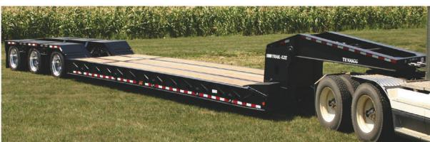
**TE110DG:** This 4 beam design has choices of 80,000 to 130,000 PSI tensile strength steel custom manufactured beams. Hydraulic non-ground bearing detachable gooseneck with air activated neck lock. Overall length is 48' on 50" axle spacing which includes 24' main deck length and 24" deck height.
