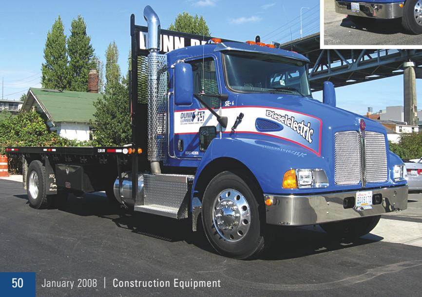
Eaton's electric hybrid drive train, depicted here in a public-utility "trouble truck," includes a 6-speed UltraShift transmission, 60-horsepower/340-lb.-ft. motor generator, two lithium-ion batteries and electronic controls.
