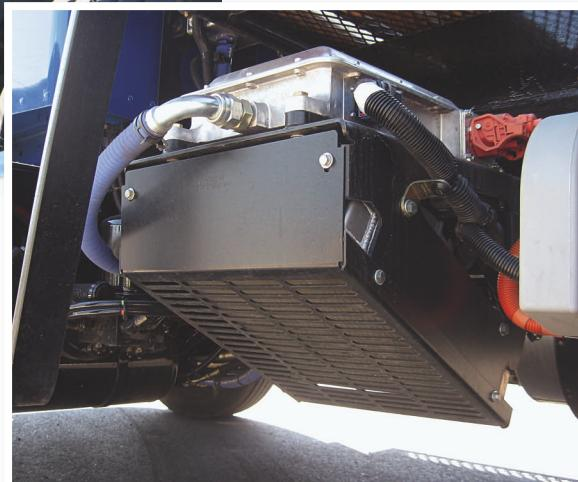
**Electronic controls (in aluminum box) sit atop cooling system, both hung on the frame behind the cab. Lithium-ion batteries are in a nearby box.**
