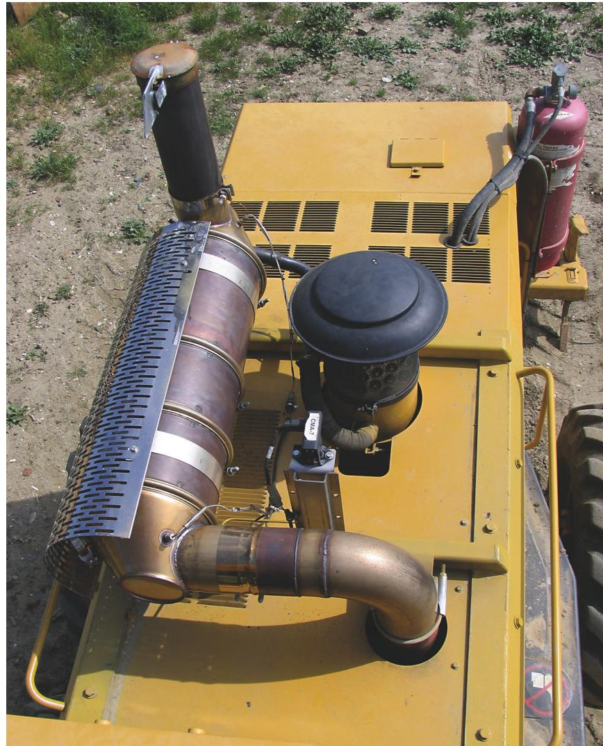
In some instances, as with Johnson Matthey's Catalyzed Continuously Regenerating Trap (CCRT), the particulate filter itself has a catalyst that promotes further production of NO<sub>2</sub>, thus supplementing the action of the DOC and potentially allowing regeneration at lower temperatures. The Donaldson Emissions Group has passively regenerated DPF units that use no DOC, only a catalyst on the filter.
