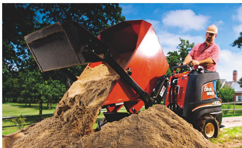
The dumper "front end" is one of seven designed to complement the 4WD versions of the R230 and R300 trenchers.
