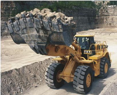
**A retrofittable Fuel Management System can reduce the 475-horsepower 988H's consumption while producing "within a few percent of maximum."**
