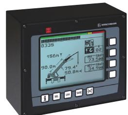
Intended for mobile crane applications, the new iVISOR mentor QGVA load moment indicator provides the operator with a graphic display of the crane as well as current load and geometric information. This includes the actual and allowable load, boom length, boom angle and load radius. The system's central processing unit and operator's console are integrated into one compact unit, making for easy installation.
