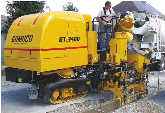
an all-new three-track footprint featuring all-track steering. This also facilitates getting on and off the stringline fast, and minimizes machine length. Powered by a 136-horsepower electronically controlled Caterpillar engine, the two-track-speed GT-3400 can travel up to 125 fpm.
