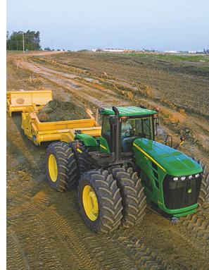
The new range of John Deere 9030-Series scraper tractors (9430, 9530 and 9630) provide horsepower ratings from 425 to 530. All three models use a John Deere PowerTech Plus diesel engine, which features exhaust-gas recirculation, variable-geometry turbocharger, up to 38-percent torque rise, and a "10-per-
