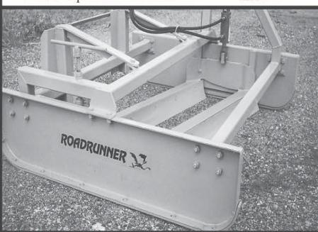
The Roadrunner has a natural tendency to run level. The long skid bar, working in combination with the dual blades, prevents dipping and gouging.
