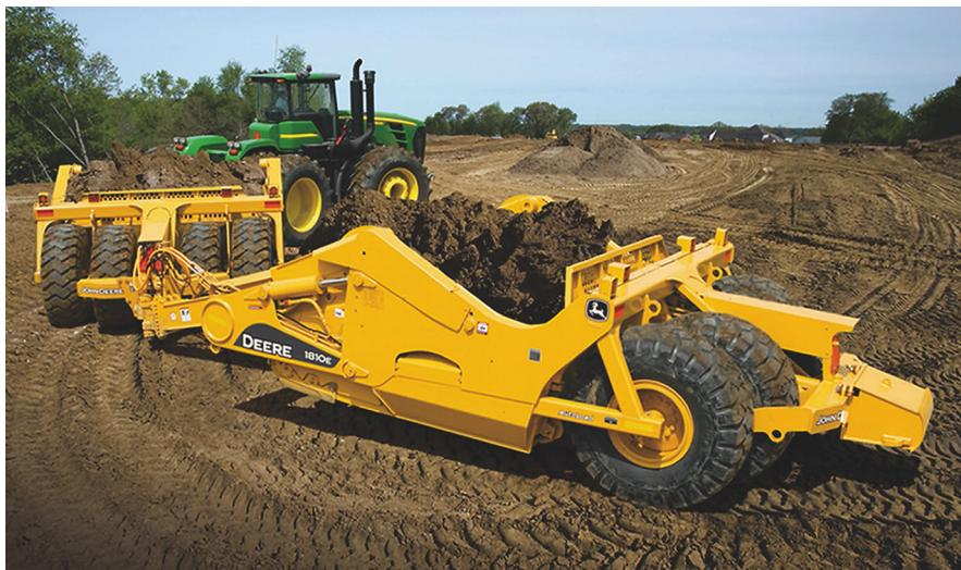
**John Deere's new 9030 Series Scraper Specials use a three-section frame, provide 15 degrees of oscillation at the articulation joint and are fitted with a 350-gallon fuel tank.**
