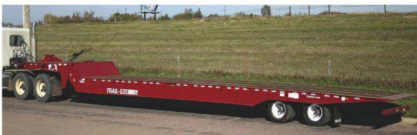
**TE701:** Heavy duty sliding axle trailer with a 6.5° load angle on the 53' long model. Patented design with 2 parallel linkage connection to the upper deck allows you to safely load the upper deck.
