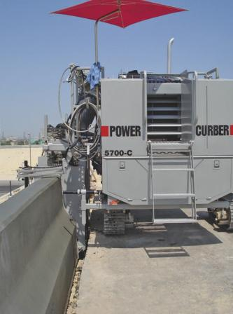
**BARRIER/PARAPET** – Walls up to 50" tall on either the left or right side of the machine.
