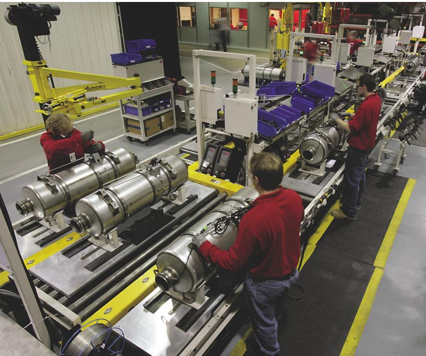
**Cummins Emission Solutions operates a manufacturing facility in Mineral Point, Wis., to manufacture diesel particulate filters, and company facilities in the United Kingdom and South Africa produce selective catalytic reduction (SCR) systems for European truck makers.**
