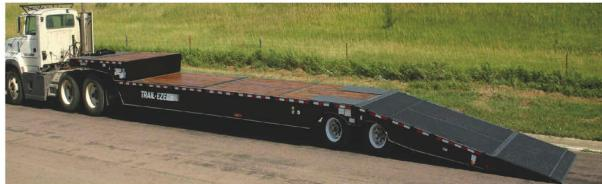
**TE70XT:** Hydraulic tail trailer with 11'3" main tail and a 5' flip tail with a low 10° load angle. The low load angle allows you to load the smallest of equipment and with the strength to load the largest. This trailer is also available with a hydraulic upper deck ramp.
